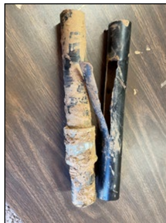
ABS plastic pipe likely broken under the weight of vehicle due to inadequate ground cover
